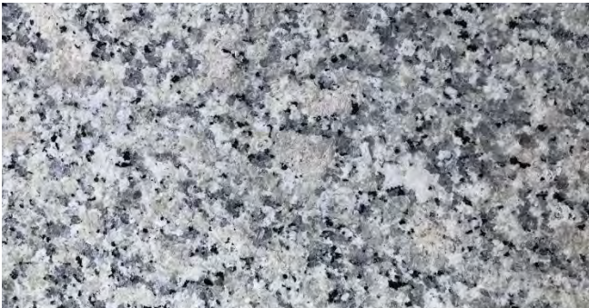
Close-up: uniform medium grained granite containing smoky quartz, plagioclase feldspar, hornblende, pyroxene
